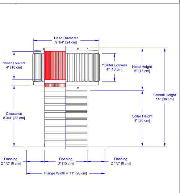
All Aluminum ConstructionMinimum Thickness = 0.025" [0.64 mm]
