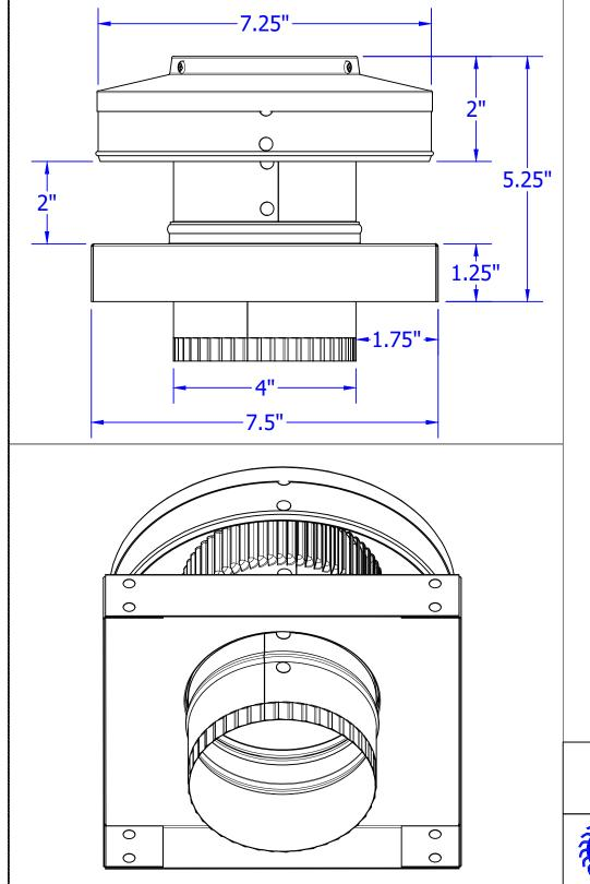
Round Back Vent with CMF & Tailpipe Model: RBV-4-C2-CMF-TP
