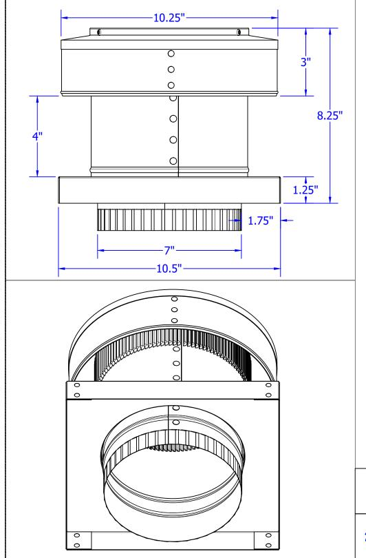
Round Back Vent with CMF & Tailpipe Model: RBV-7-C4-CMF-TP
