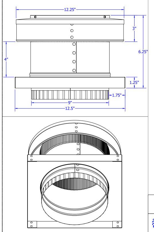
Round Back Vent with CMF & Tailpipe Model: RBV-9-C4-CMF-TP
