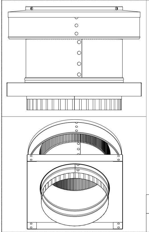
Round Back Vent with CMF & Tailpipe Model: RBV-9-C4-CMF-TP
