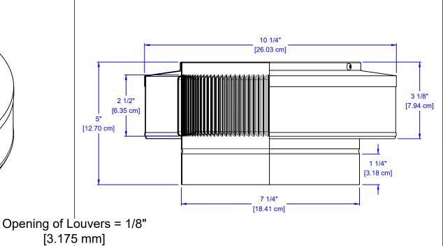
All Aluminum Construction Thickness = 0.025" [0.635 mm]
