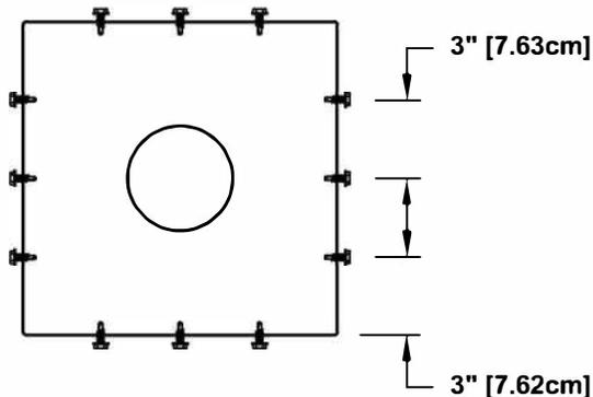
Roof Vent with Curb Mount Flange accessory
