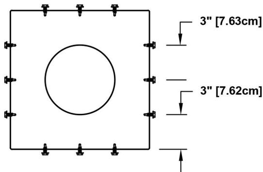
Roof Vent with Curb Mount Flange accessory
