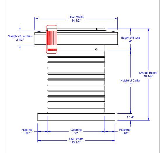
Aluminum Alloy 3000 Series Minimum Material Thickness = .025" ± .005"
