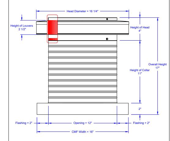
Aluminum Alloy 3000 Series Minimum Material Thickness = .025" ± .005"
