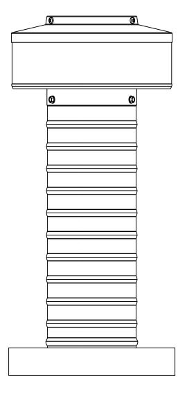
Aluminum Alloy 3000 Series Minimum Material Thickness = .025" ± .005"
