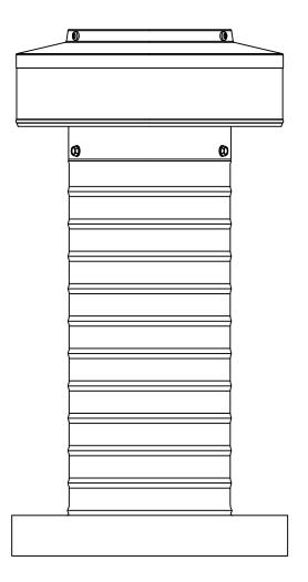
Aluminum Alloy 3000 Series Minimum Material Thickness = .025" ± .005"
