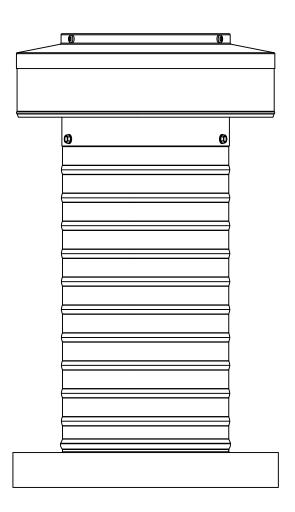
Aluminum Alloy 3000 Series Minimum Material Thickness = .025" ± .005"
