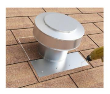
10A: Required screw: #10 x 1.5" steel sheet metal screw Total number of screws required = 8
