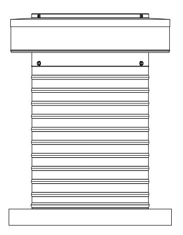
Aluminum Alloy 3000 Series Minimum Material Thickness = .025" ± .005"
