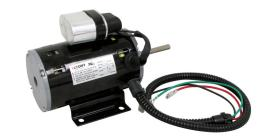
Replacement motors for AVP's 14 inch diameter fans. A Permanent Split Capacitor (PSC) Motor is a type of single-phase AC motor. More specifically, a type of split-phase induction motor in which the capacitor is permanently connected as opposed to only being connected when starting. The motor is 3.3 inches in diameter and is mainly for HVAC applications such as inline fans.
