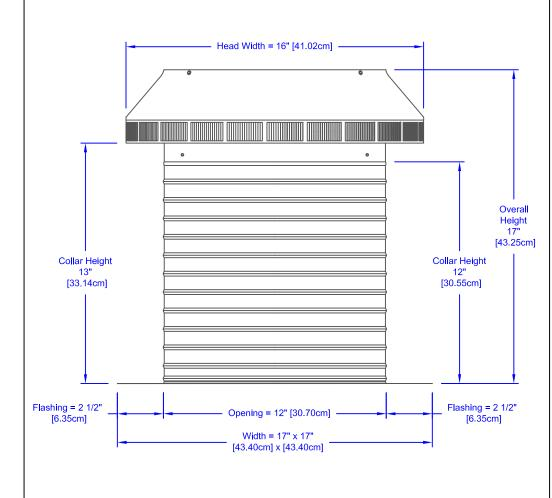
All Aluminum Construction, Thickness = 0.025" [0.635 mm]
