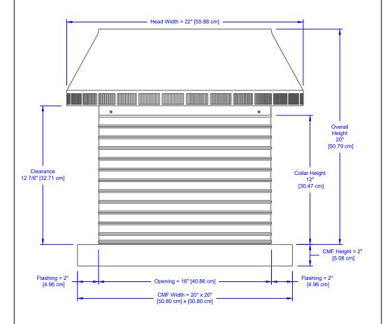
All Aluminum Construction, Thickness = 0.040" [1.016 mm]
