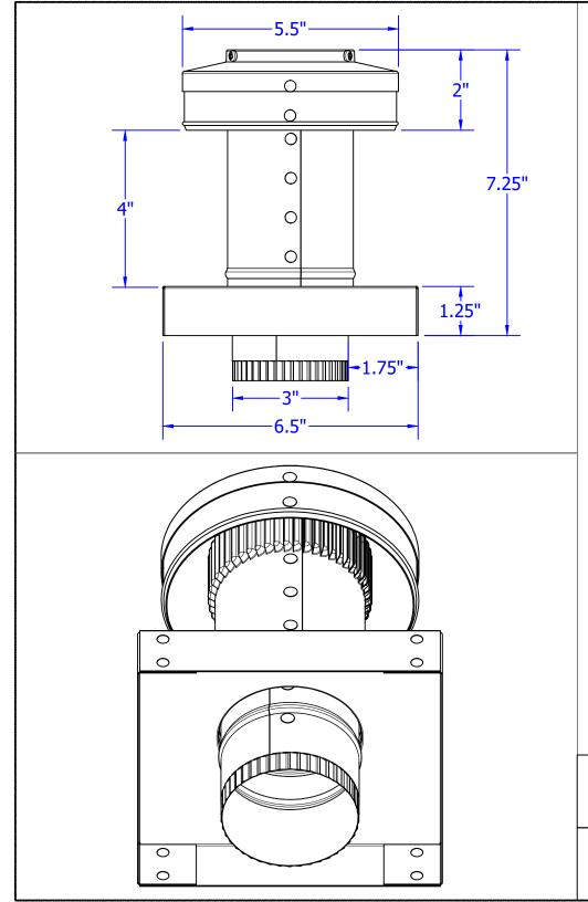
Round Back Vent with CMF & Tailpipe Model: RBV-3-C4-CMF-TP
