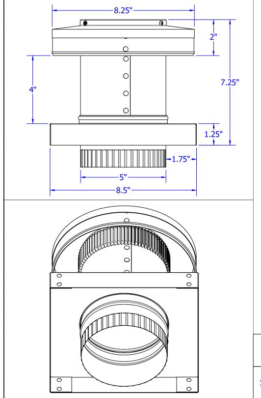
Round Back Vent with CMF & Tailpipe Model: RBV-5-C4-CMF-TP
