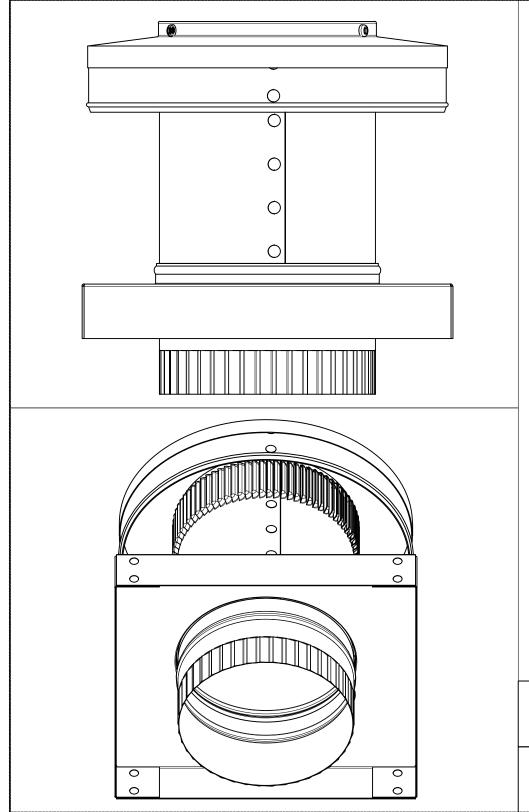
Round Back Vent with CMF & Tailpipe Model: RBV-5-C4-CMF-TP
