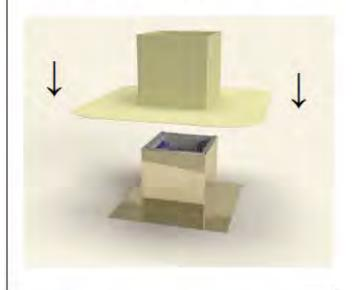
Step 12: Install roof vent, exhaust fan or pipe cap over curb using recommended screw. See appropriate Vent with Curb Mount Flange installation instructions at roofvents.com for more details.
