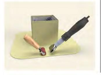
Step 10: Drop down the TPO boot over the roof curb.
