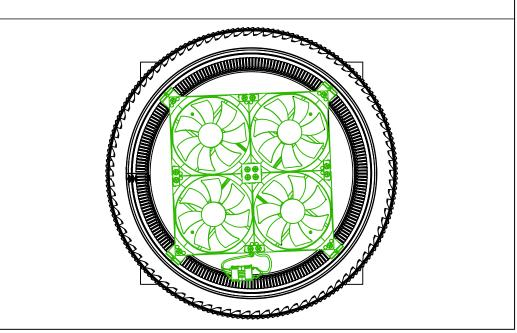
Aura Solar Attic Fan with CMF Model: ASF-14-C4-CMF Diameter: 14" Collar Height: 4"
